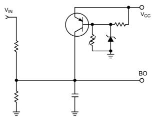
Figure 4. How to Perform a Latched OTP or OVP
