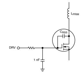
Figure 14. Gate-to-Ground Capacitor
