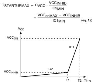
Figure 16. Dual Startup Current Source
