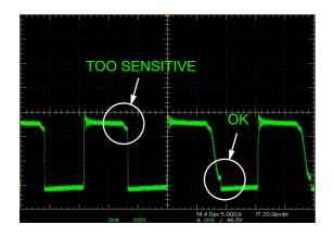
Figure 13. Instability with Multiple Outputs
