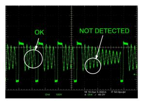
Figure 11. Instability at Lower Load
