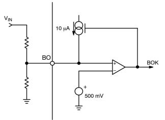
Figure 2. Internal Configuration of BO Protection
