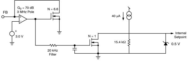
Figure 5. Internal Circuitry of FB Pin
