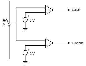
Figure 3. Internal Implementation of Disable and Latch Comparators
