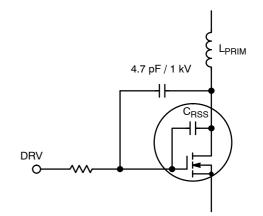
Figure 12. External Gate-to-Drain Capacitor
