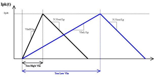
Figure 7. T<sub>ON</sub> Behavior at a Biven  $I_{pk}$  for Different V<sub>IN</sub>
