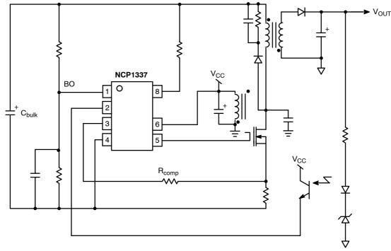
Figure 1. NCP1337 Typical Application Example
