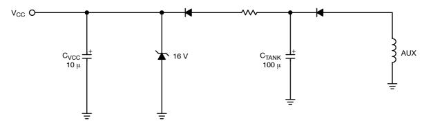
Figure 18. Split Capacitor on V<sub>CC</sub> Pin
